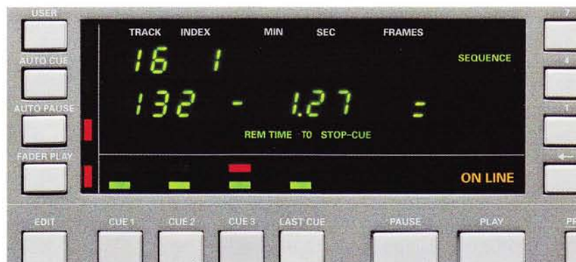
CD player in sequence function CUE 1-3-2. Indication of the remaining time to the end of the sequence: 1 Min 27 Sec. Currently CUE 3 is being played.
