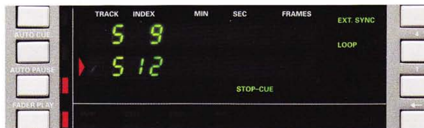
For sound effects e.g. any STOP CUE can be defined. In «jingle play mode», the laser returns to the START CUE when the STOP CUE is reached and waits there in pause mode.
